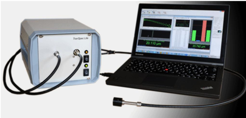
The **TranSpec Lite** film thickness gauges use the white-light interference phenomenon for non-contact and non-destructive layer determination of transparent single or double layers in the range of around 0.8 to 120 micrometers (depending on the model). The TranSpec Lite instruments are designed for manually performed, but even though high-precise measurements in the lab.
